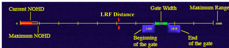
Figure 7: Range-gate cursor and indicator
