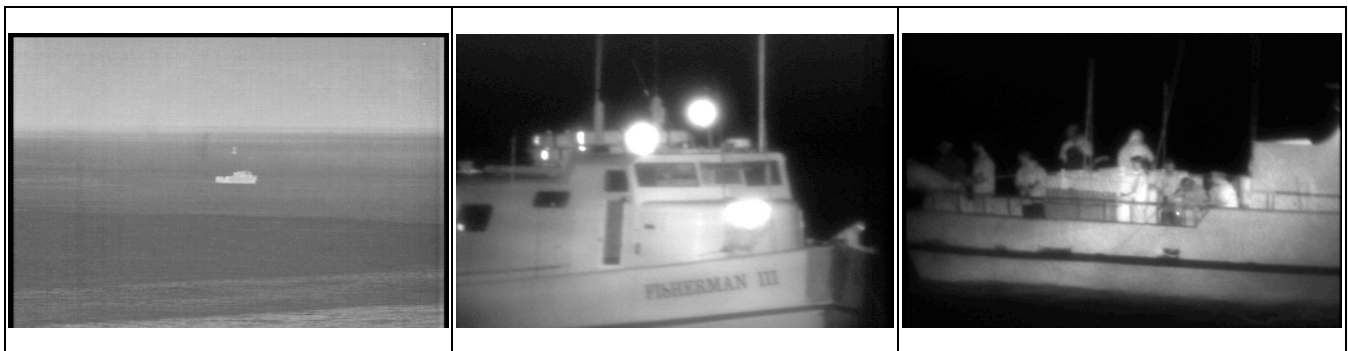
Figure 3: A fishing boat at 1,9 km seen by a thermal imager (a) and the ATV-2000i (b and c)
