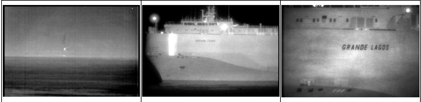
Figure 4: A large ship at 6,4 km as seen by a thermal imager (a) and by the ATV-2000i (b and c)
