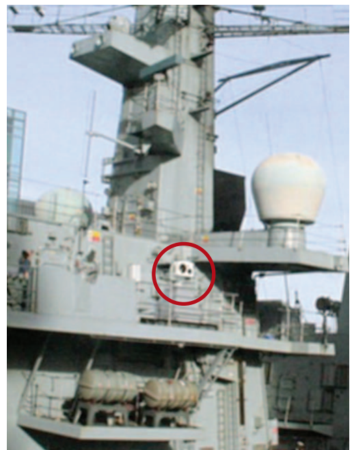
ARGC-2400 mounted on a gyro stabilized platform deployed on a frigate
