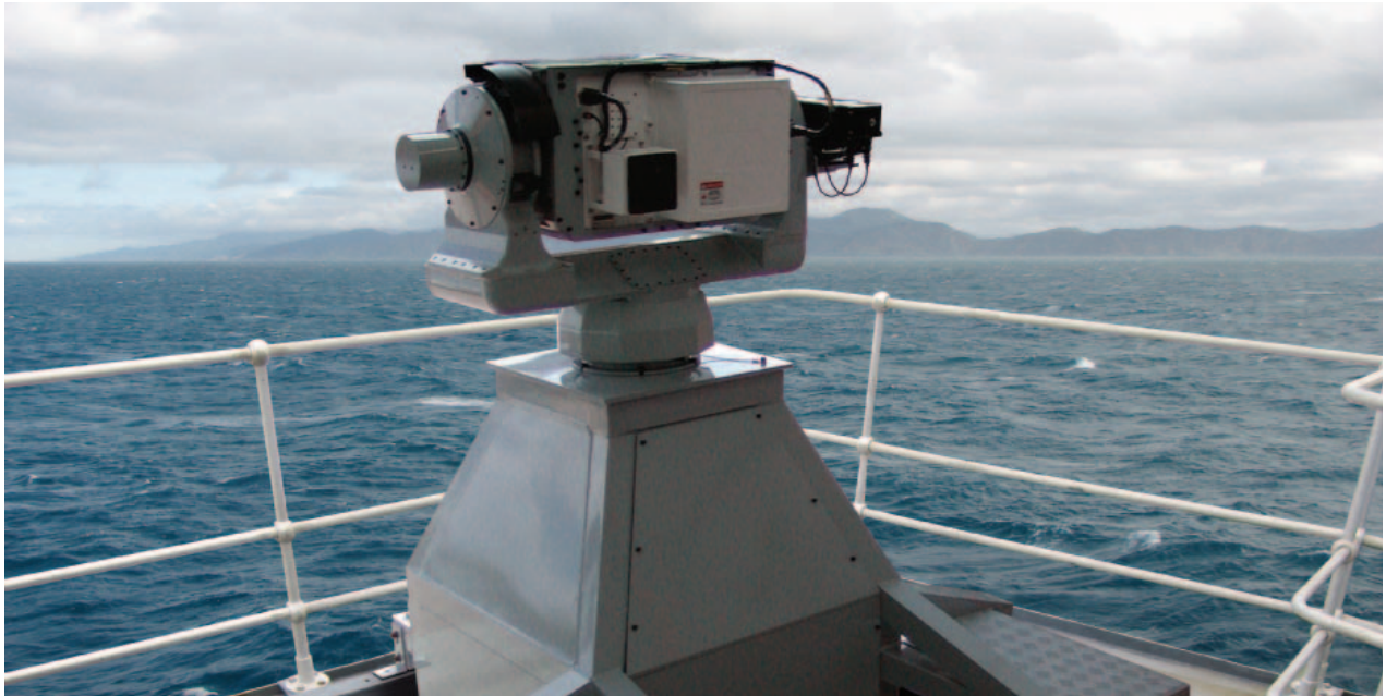
Positioner with suggested mounting plinth
