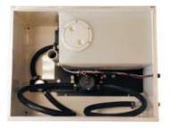
The water tank contains 30 L and the pump has a capacity of 14.3 L per min.
